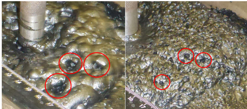
Figure 7. Example of local bubble collapses from the froth images during coal flotation.
