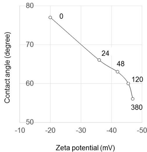
**Figure 1.** Contact angle and zeta potential of oxidized bituminous coal. Numbers next to the plots indicate the oxidation time (h) at 125 °C (reproduced from [16]).
