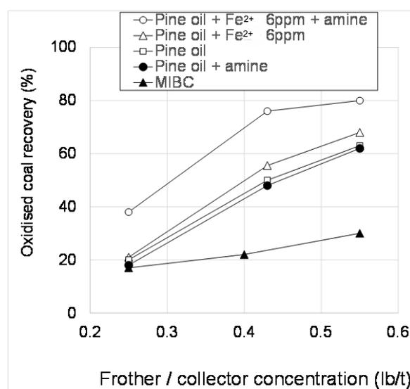
**Figure 2.** Effect of frother, amine and ferrous ions on the flotation recovery of oxidized coal at pH 6.5 (reproduced from [16]).
