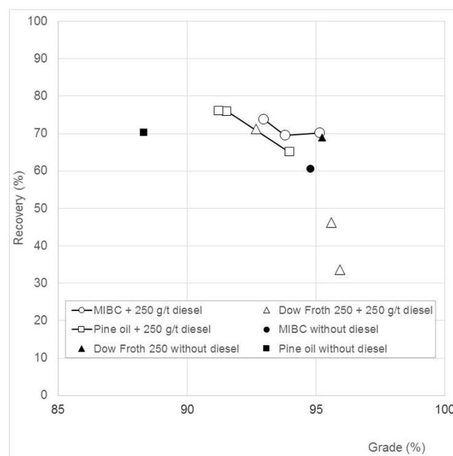
**Figure 3.** Grade – recovery curve of coal flotation tests with 3 different frothers in the absence or presence of 250 g/t diesel collector (adapted from [27]).
