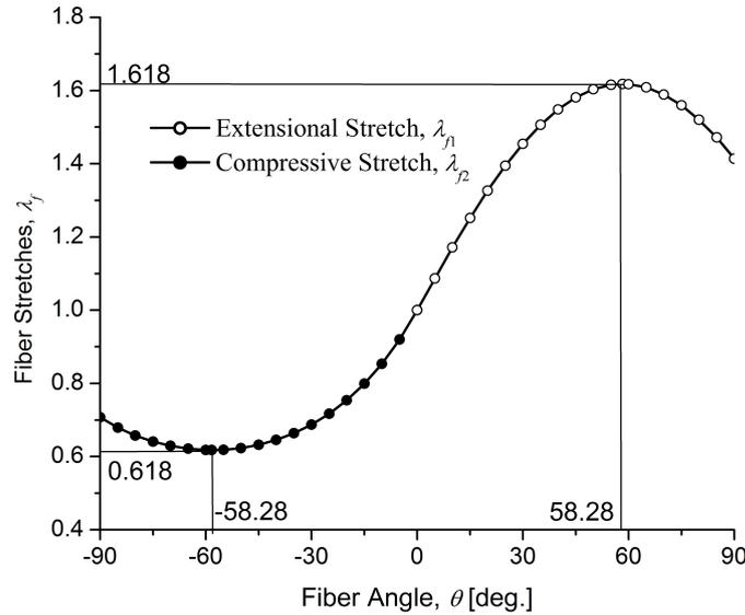
**Figure 2.** Fiber stretches as function of fiber angle with  $\kappa_m = 1$  in simple shear deformations.
