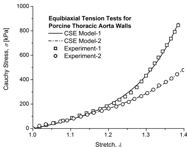
**Figure 4.** Comparison between CSE models and equibiaxial tension tests for porcine aortas.
