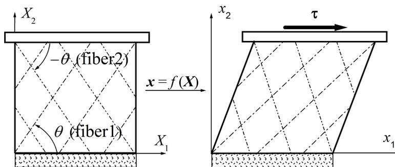
Figure 1. Simple shear tests of unit cube with two families of in-plane fibers.
