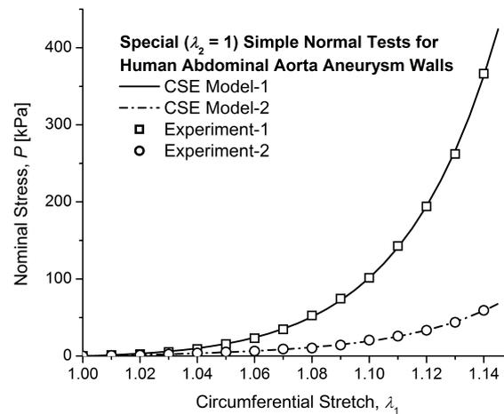
**Figure 5.** Comparison between CSE models and special simple normal tests for human AAAs.
