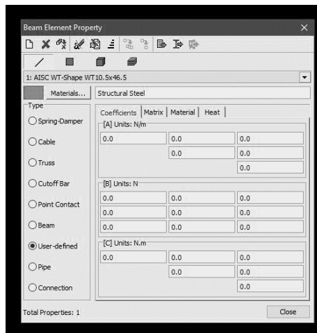
Figure 7. Strand7 Input Panel for aprismatic beams
