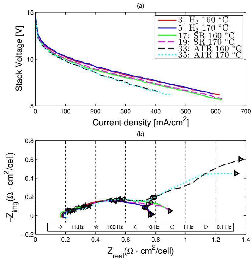
**Figure 19.** Impedance plots comparing for dry H<sub>2</sub>, SR gas and ATR gas operation modes at 160 °C and 170 °C
