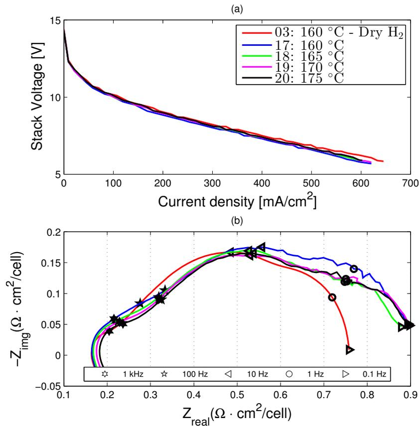
Figure 7. Temperature test under reformate gas operation
