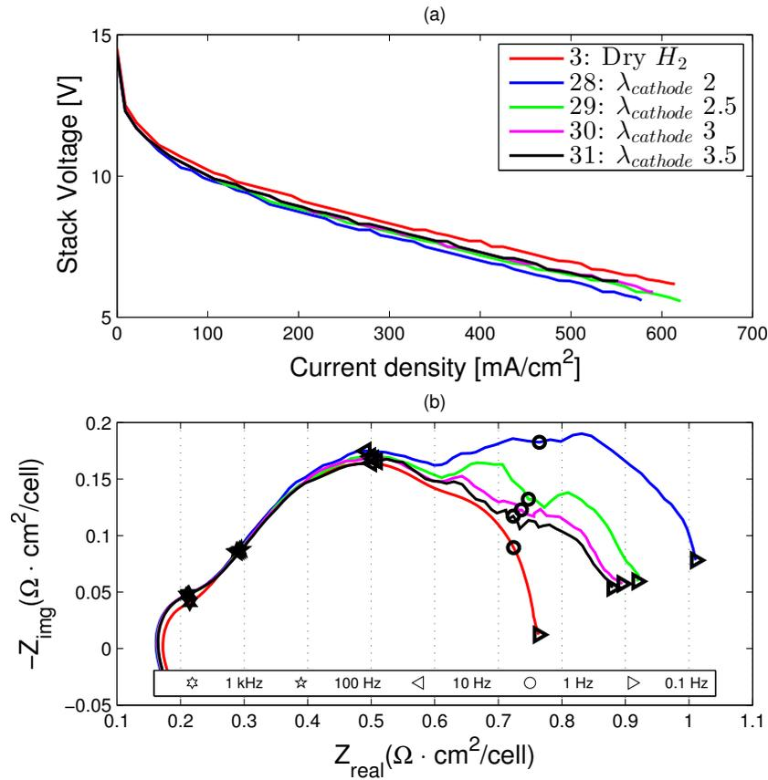
Figure 15. Impedance plot at different air stoichiometry levels under SR gas operation
