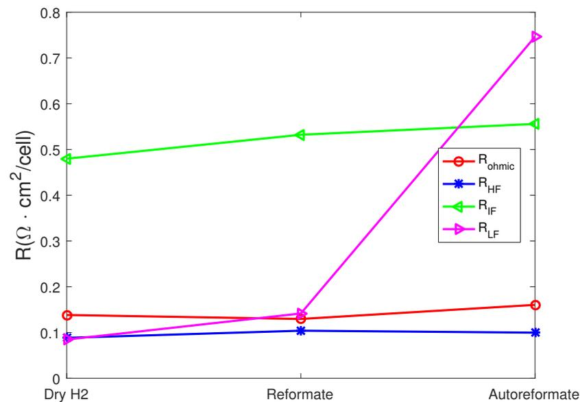
**Figure 20.** Comparison of dry H<sub>2</sub>, SR gas and ATR gas operation modes at 160 °C
