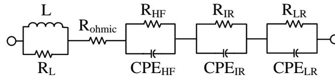
**Figure 3.** EC model representation of HT-PEMFC stack used in this work
