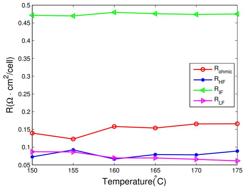
Figure 6. Effects of temperature under dry H<sub>2</sub> operation
