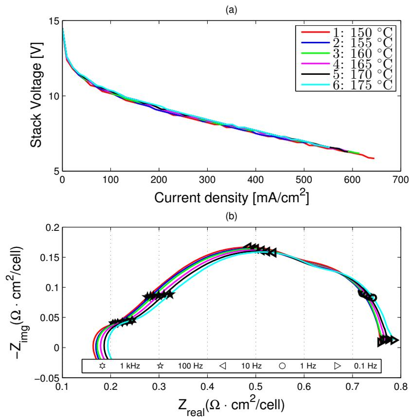
Figure 5. Effects of temperature under dry H<sub>2</sub> operation
